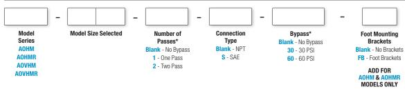
AOHMR - Internal pressure bypass included
